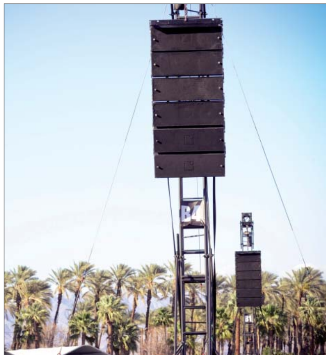
5- Two of the V-DOSC delay arrays to support the Main Stage system
