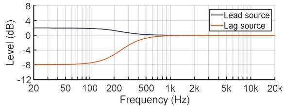
Figure 3. Frequency response of the LF contour modifications applied to the lead and lag sources.
