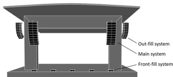
Figure 1. Illustration of typical main and fill loudspeaker systems deployed on a stage.
