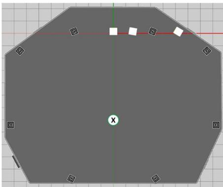
Figure 4. Top view of loudspeaker setup and listening position (white squares represent loudspeakers fed by dry signals, black squares are reverb loudspeakers).
