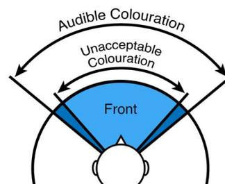
Figure 2. Illustration of audible and unacceptable coloration areas resulting from the combination of a lead source at 0° and a lag source at -6 dB (from [11]).
