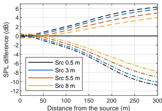
**Fig. 9:** SPL difference between downwind and no wind conditions (dashed line) and between upwind and no wind conditions (dash-dotted line), ground roughness length 0.1 m.
