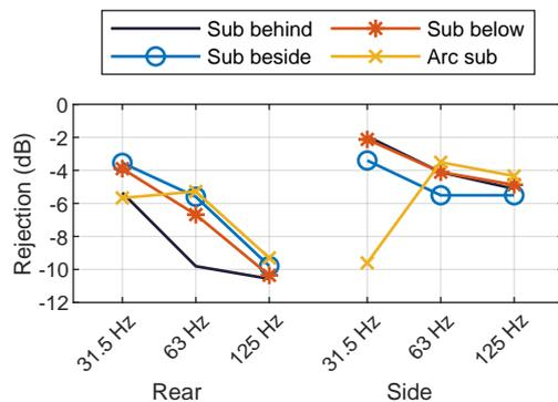
**Fig. 7:** SPL rejection at the rear and on the sides of the system, at 1000 m, in octave centered at 31.5 Hz, 63 Hz, and 125 Hz, for several subwoofer configurations.
