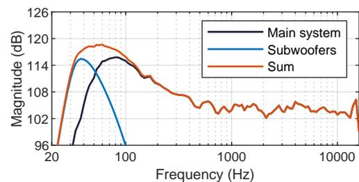
**Fig. 1:** Typical frequency response of a full-range system (L-Acoustics K2), subwoofers (L-Acoustics KS28) and the sum of both.
